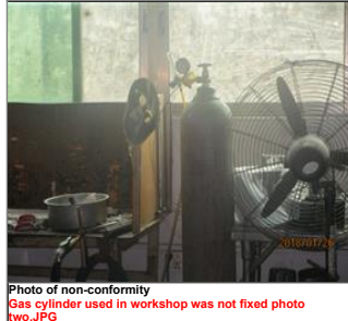
Photo of non-conformity Gas cylinder used in workshop was not fixed photo one.JPG
